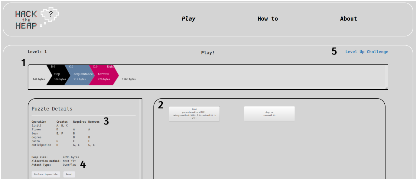
Fig. 2: A screenshot of the heap puzzle game being played. The numbers correspond as follows: 1. is the playing board (or heap memory space if you like). 2. shows all operations that can be performed at the current stage of the game. 3. shows all requirements of operations before said operation can be used. 4. shows additional details about the puzzles. 5. is a link to the tutorial where the player can level up.
